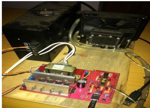
Figure A.1. Bovine's semen temperature control hardware
