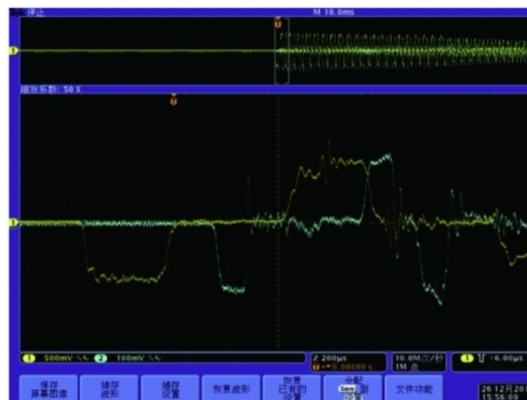
Fig. 23. The Original waveform curve under 3000 \text{ s}^{-1} strain rate. The photos of fracture specimens of high nitrogen steel are shown in Fig. 24.
