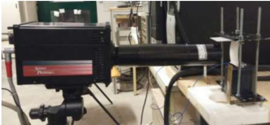
Figure: 3.2: Test bench, infrared camera and zoom setup.
