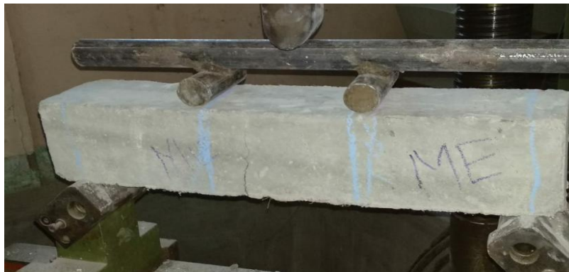
Fig 3: Flexural Strength Test
