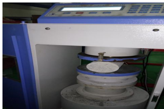
Fig 2: Split Tensile Strength Test
