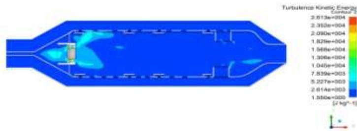
**Fig 13.0** Contour of turbulent kinetic energy, case 2
