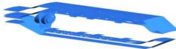
Fig 2.0 Combustion chamber without dilution tubes
