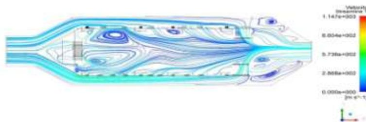
Fig 10.0 Streamlines in combustor, Case 2
