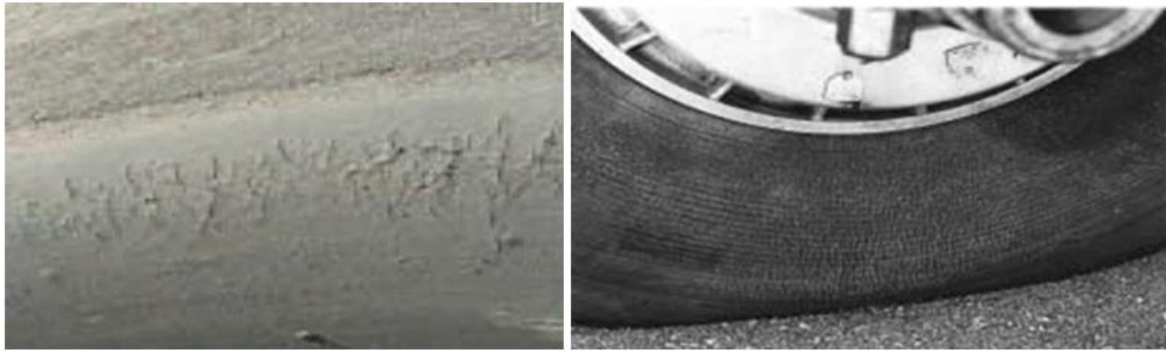
Figure 2 Surface cracks on the tyres (Source: Michelin and Goodyear)
