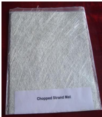
Figure. 1 Chopped Strand Mat Fabric
