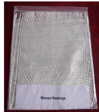
Figure. 3 Woven Rovings Fabric
