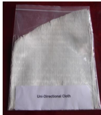
Figure. 2 Uni-Directional Cloth Fabric
