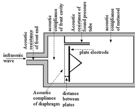
Fig. 2. Work principle diagram of CASI-ISM-2013 infrasound sensor.
