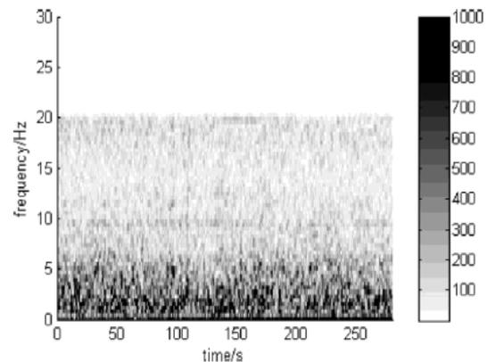
Fig. 4. Time-frequency diagram of environmental noise signal (Grayscale represents the size of the intensity).
