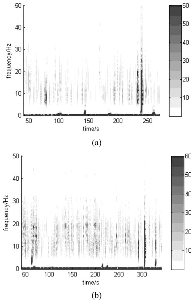
Fig. 6. The time-frequency diagrams of infrasonic wave (Grayscale represents the size of the intensity).
