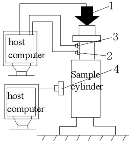
1. Axial compression system; 2. Stress transducer; 3. strain transducer; 4. acquisition system of infrasonic wave.
