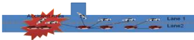
Fig 2: Dissemination of road side construction information to the vehicles of targeted areas through V2V communication.
