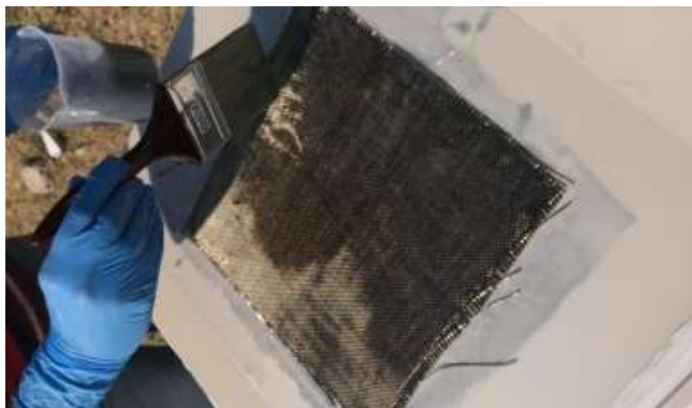
FIGURE 1 HAND LAYUP METHOD
