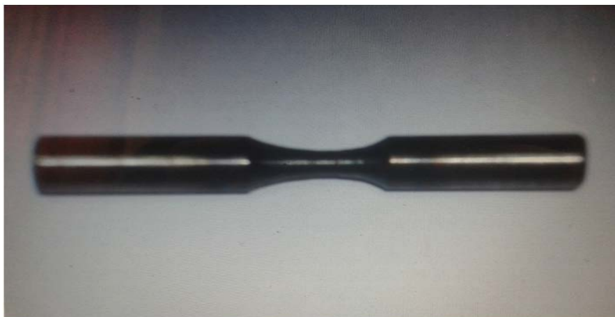
Fig. (2): Sample number (2) after hardening
