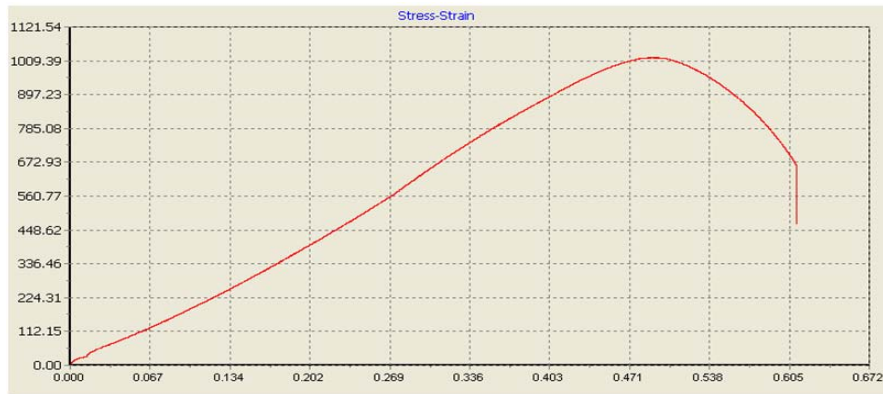
Fig. (3) stress-strain curve of a tensile test sample
