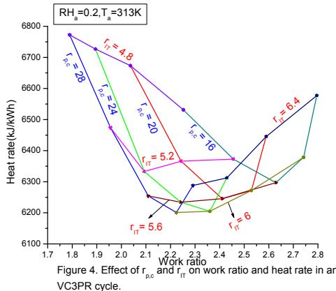
Figure 4. Effect of  $r_{p,c}$  and  $r_{IT}$  on work ratio and heat rate in an VC3PR cycle.
