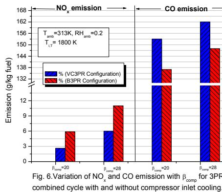
Fig. 6. Variation of  $NO_x$  and CO emission with  $\beta_{comp}$  for 3PR combined cycle with and without compressor inlet cooling.
