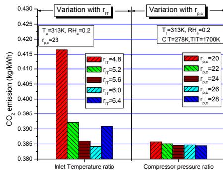
Figure 5. Variation of CO<sub>2</sub> emission with  $r_{IT}$  and  $r_{p,c}$  for VC3PR cycle
