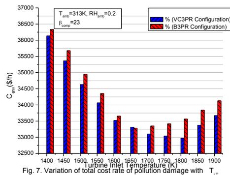
Fig. 7. Variation of total cost rate of pollution damage with  $T_{i,T}$  of 3PR cycle with and without compressor inlet cooling.
