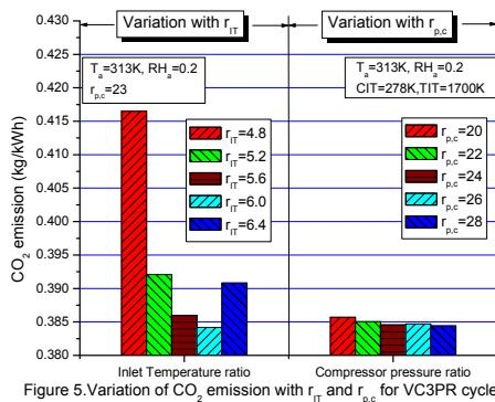
Figure 5. Variation of  $CO_2$  emission with  $r_{IT}$  and  $r_{p,c}$  for VC3PR cycle
