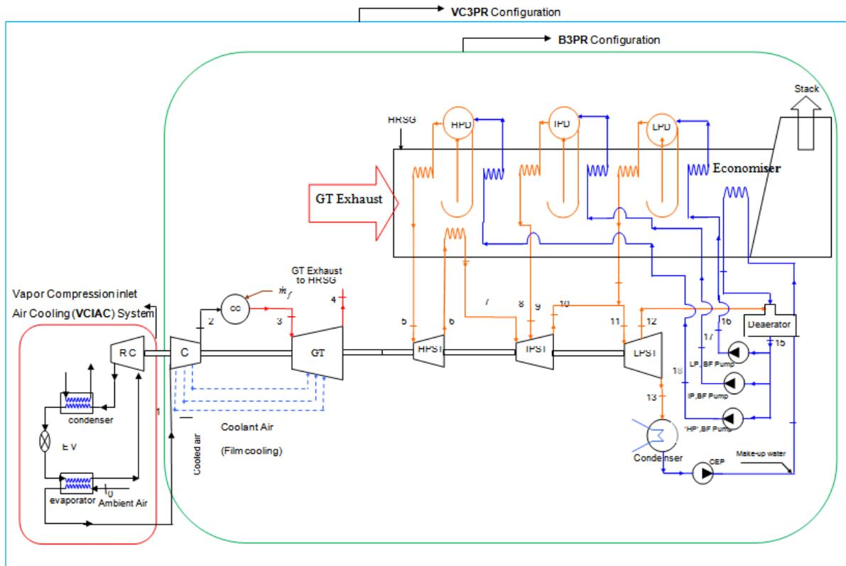
A vapor compression refrigeration cycle has been used to cool the compressor inlet air. The work of refrigeration needed for cooling the inlet air has been extracted from the gas turbine output. The actual power required to run the refrigeration system is more than the theoretical power due to various associated losses. So the actual refrigerating compressor power is given by
