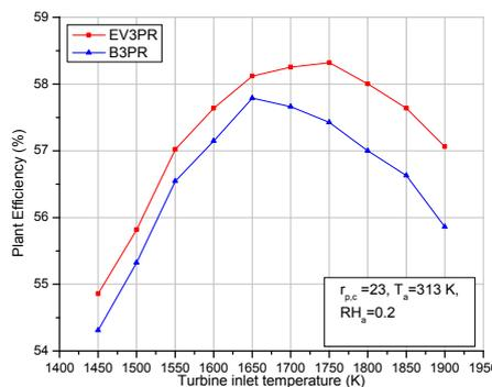
Fig.3. Variation of plant efficiency with TIT for 3PR cycle with and without inlet air cooling
