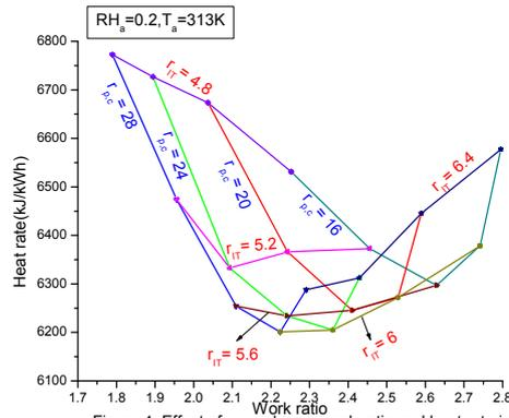
Figure 4. Effect of  $r_{p,c}$  and  $r_{IT}$  on work ratio and heat rate in an VC3PR cycle.
