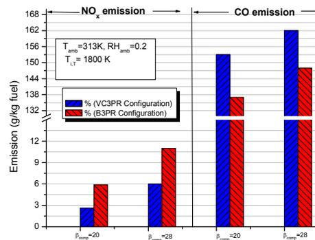
Fig. 6. Variation of NO<sub>x</sub> and CO emission with  $\beta_{comp}$  for 3PR combined cycle with and without compressor inlet cooling.
