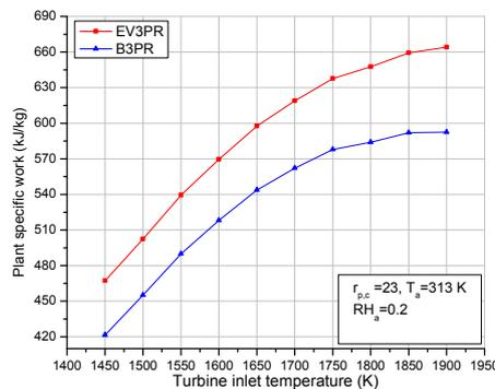
Fig.2. Variation of plant specific work with TIT for 3PR cycle with and without inlet air cooling
