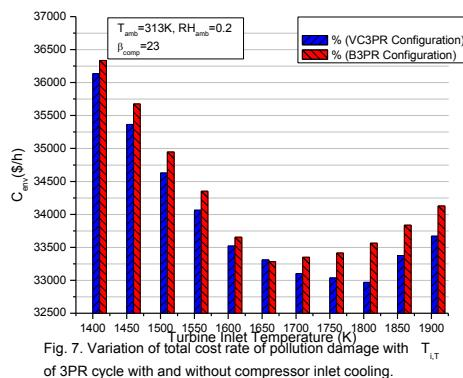
Fig. 7. Variation of total cost rate of pollution damage with  $T_{i,T}$  of 3PR cycle with and without compressor inlet cooling.
