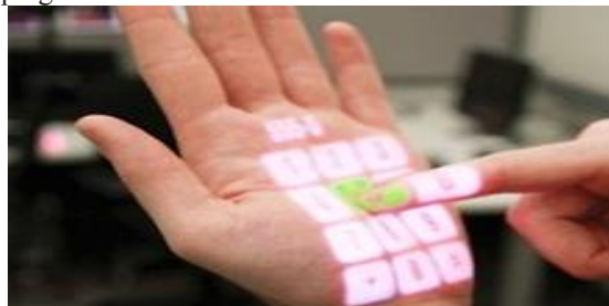
Figure 1: Skinput uses bio-acoustic sensor and sophisticated machine learning to turn the human palm into a touch pad.
