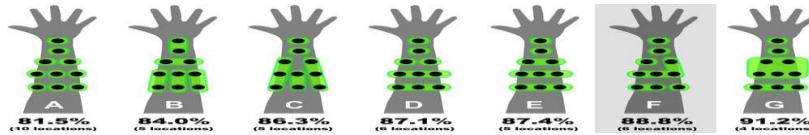
Figure 9: Higher accuracies can be achieved by collapsing the ten input locations into groups. A-E and G were created using a design-centric strategy. F was created following analysis of per-location accuracy data. As per study conducted at Carnegie mellon university by Chris Harrison, Desney tan, Dan morris.
