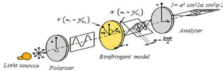
**Figure 2:** Light propagation through a photoelastic model
