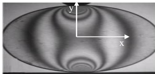
**Figure 3:** Isochromatics fringes obtained on the disc
