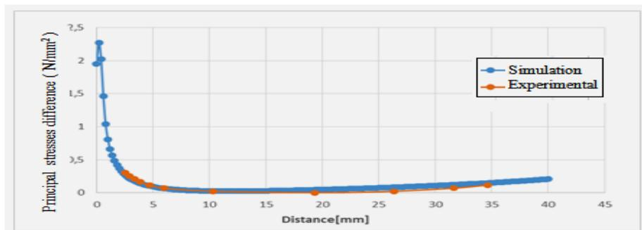
**Figure 9:** Principal stresses difference along the vertical axis osymmetry
