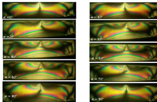
**Figure 6:** Isoclinics recorded for different polarizer and analyzer positions
