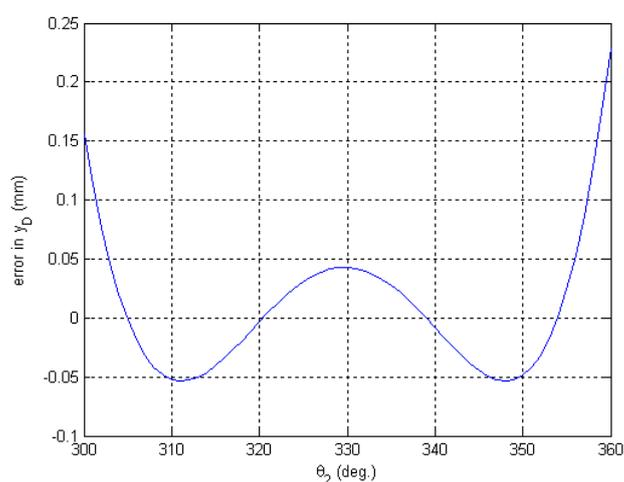
Fig.6: Error in the slider displacement.
