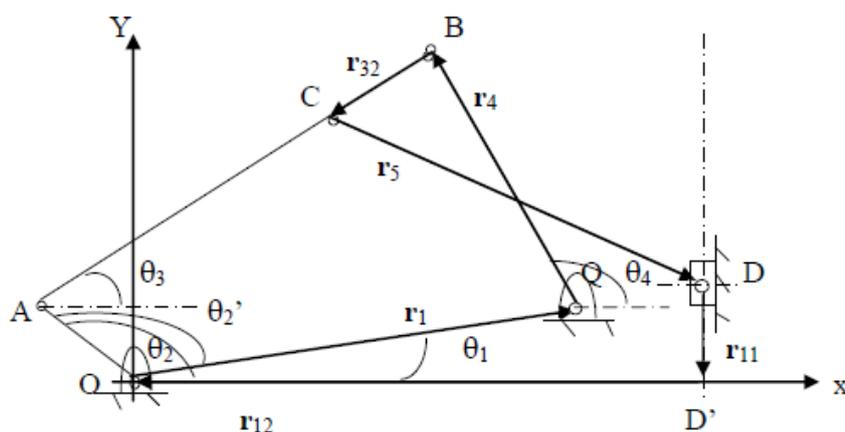
Fig.2: Displacement analysis of the 6-bar dwell mechanism.
