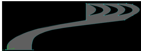
Fig. 1.9: Solid Model as a Partial Admission Case of Nozzle and Rotor Blades with 5mm axial gap.
