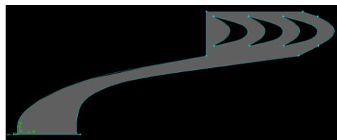
Fig 1.8: Solid Model as A Partial Admission Case of Nozzle and Rotor blades with 4mm axial gap.
