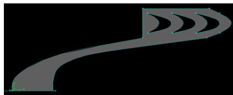
Fig. 1.7: Solid Model as a Partial Admission Case of Nozzle and Rotor Blades with 3mm axial gap.
