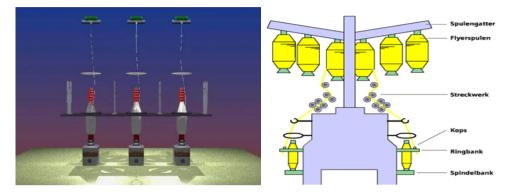
Fig.12 Diagram of Twisting System
