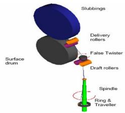
Fig. 13 Diagram of Ring spinning frame
