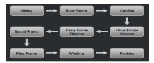
Fig. 1 Diagram of yarn manufacturing process
