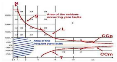
Fig. 17 Diagram of Yarn fault classes
