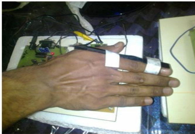
Figure 3.3 : FLEX sensor attached to the finger of human
