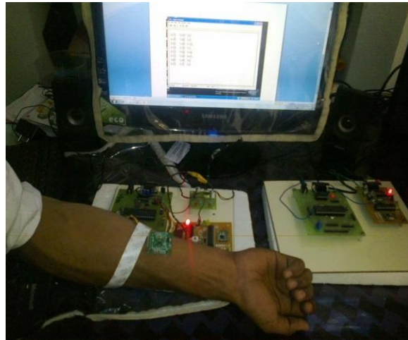
Figure 3.2: MEMS Sensor attached to the human
