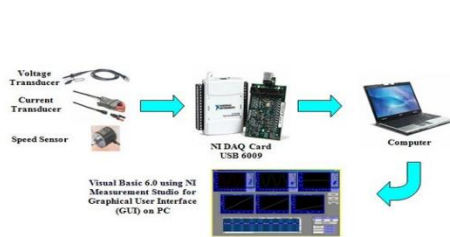
Fig 1.2: Monitoring of motor using DAQ Motor Monitoring
