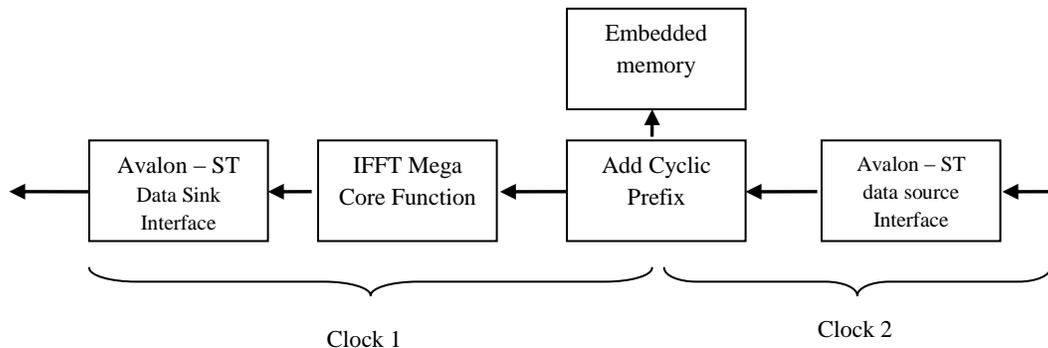
Figure5. Uplink OFDM Kernel Block Diagram
