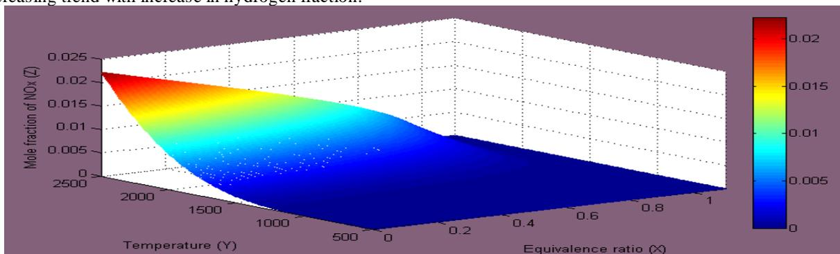
**Fig.6:** Effect of Temperature and equivalence ratio on mole fraction of  $\text{NO}_x$
