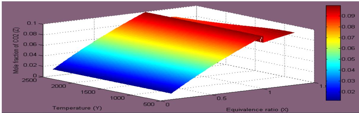
**Fig.4:** Effect of equivalence ratio and temperature on the mole fraction of  $\text{CO}_2$  at  $x=0.3$
