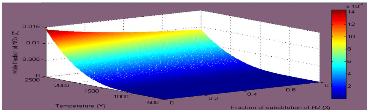
**Fig.5:** Effect of Temperature and Hydrogen fraction on mole fraction of  $\text{NO}_x$  at  $\text{equ}=0.6$
