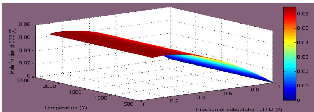
**Fig.3:** Variation of Mole fraction of CO<sub>2</sub> with change in Temperature and Hydrogen fraction at  $\phi=0.3$
