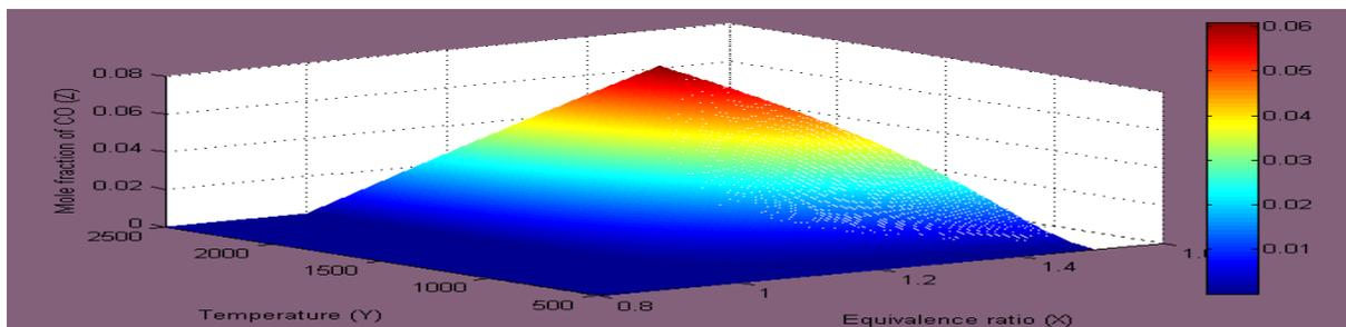
**Fig.2:** Effect of Temperature and equivalence ratio on mole fraction of CO for  $\phi=0.3$
