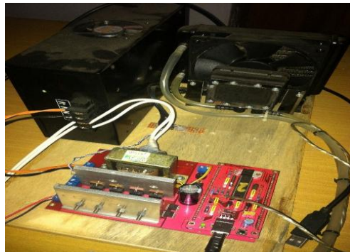
Figure A.1. Bovine's semen temperature control hardware
