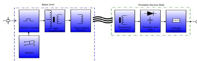
The concept of wireless electricity works on the principle of using coupled resonant objects for the transfer of electricity to objects without the use of any wires. This concept of WiTricity was made possible using resonance where an object vibrates with the application of a certain frequency of energy. So two objects having similar resonance tend to exchange energy without causing any effects on the surrounding objects.
