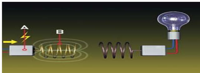
A circuit [A] attached to the wall socket converts the standard 60-hertz current to 10 megahertz and feeds it to the transmitting coil [B]. The oscillating current inside the transmitting coil causes the coil to emit a 10-megahertz magnetic field
