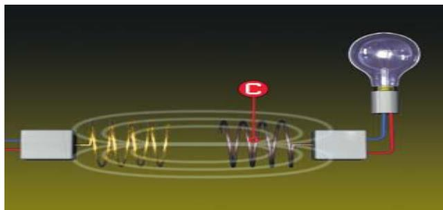
The receiving coil [C] has the exact same dimensions as the sending coil and thus resonates at the same frequency and, in a process called magnetic induction, picks up the energy of the first coil's magnetic field.
