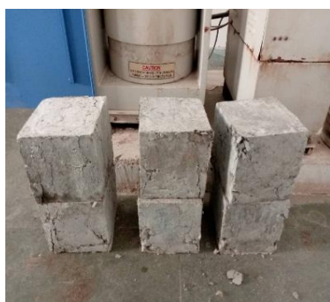
Fig. 14: Cube after Testing.
