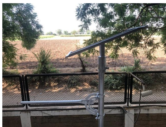
Fig. New Design of solar LED street light
