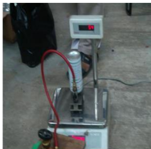
b) charging of the refrigerant
