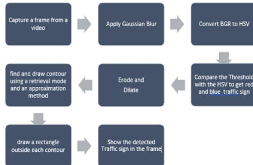
**BlockDiagram of Traffic Sign Detection with CNN**
