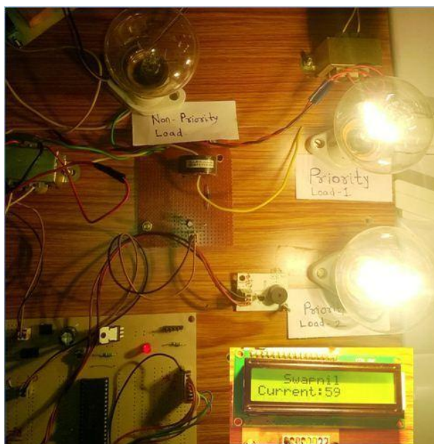
Fig.10. Stable system after non-priority load Trimming
