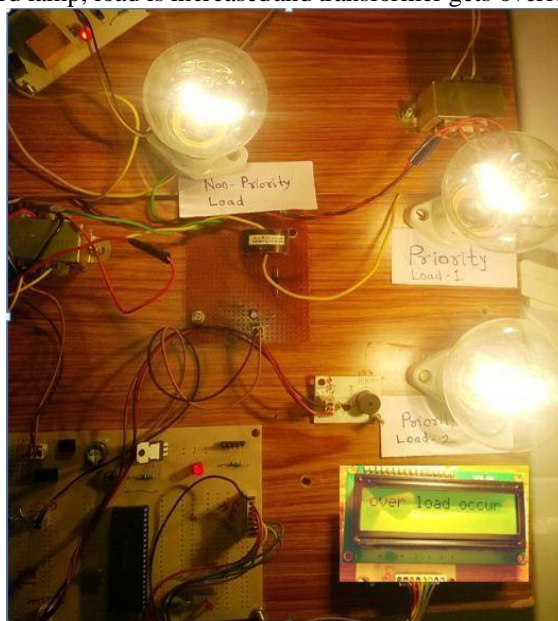
Fig.9. Over load condition of Transformer
