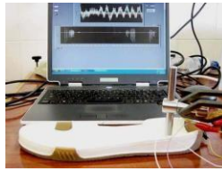
Fig. 10 Performance test. A handspike system was used in order to apply constant pressure impulses to the sole.
