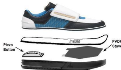
Fig. 2 First prototype of the energy generator. Two piezoelectric polymer films above the sole.
