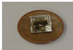
Fig. 7. Circuit implemented in the final prototype shown on a 1-cent Euro coin.
