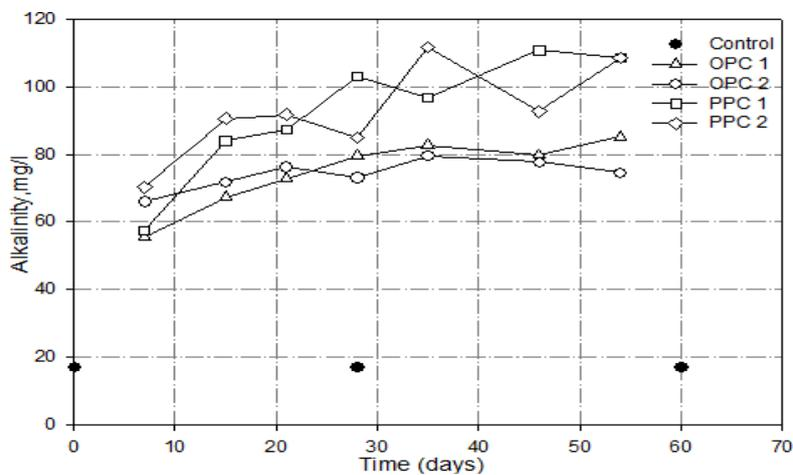
Figure 3 Variation of Alkalinity of stored rainwater with time
