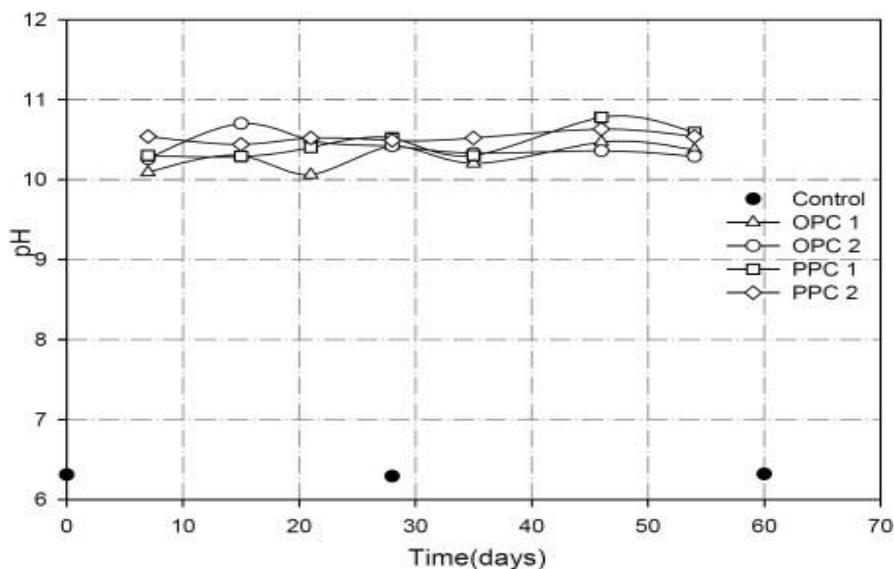
Figure 2 Variation of PH of rainwater on storage
