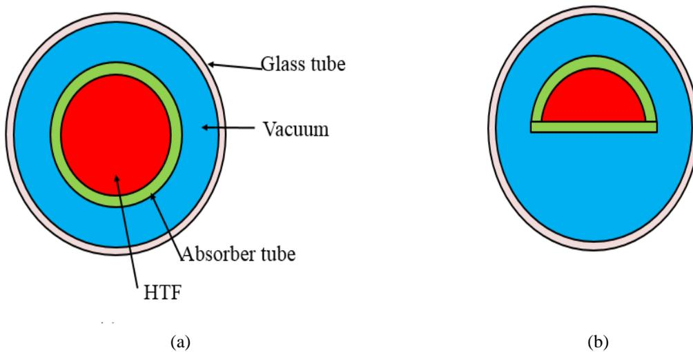
Fig. 2 Cross sectional view of receiver (a) circular absorber tube (b) semicircular absorber tube
