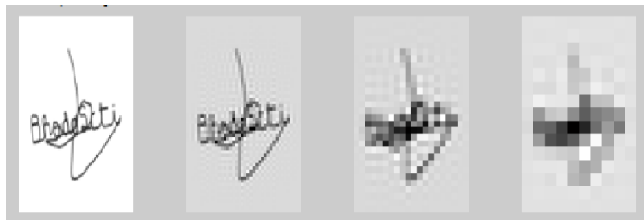
Figure 3: Results of Gaussian pyramid of level 1, 2, 3 respectively
