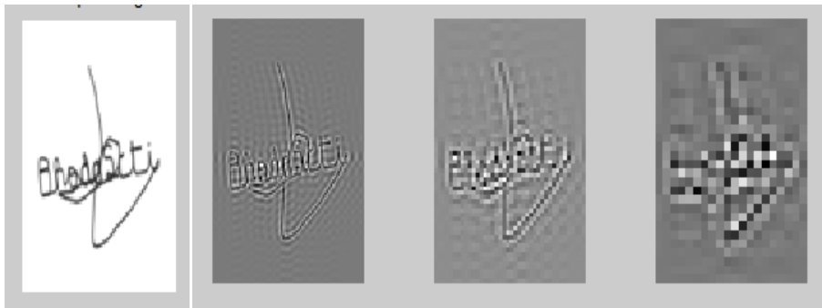
Figure 4: Results of Laplacian pyramid level 1, 2, 3 respectively
