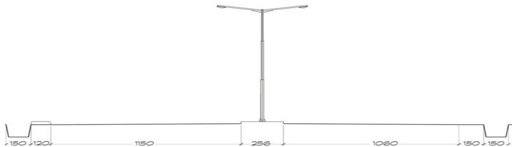
Figure 2. Sectional Crossing on Urip Sumohardjo road
