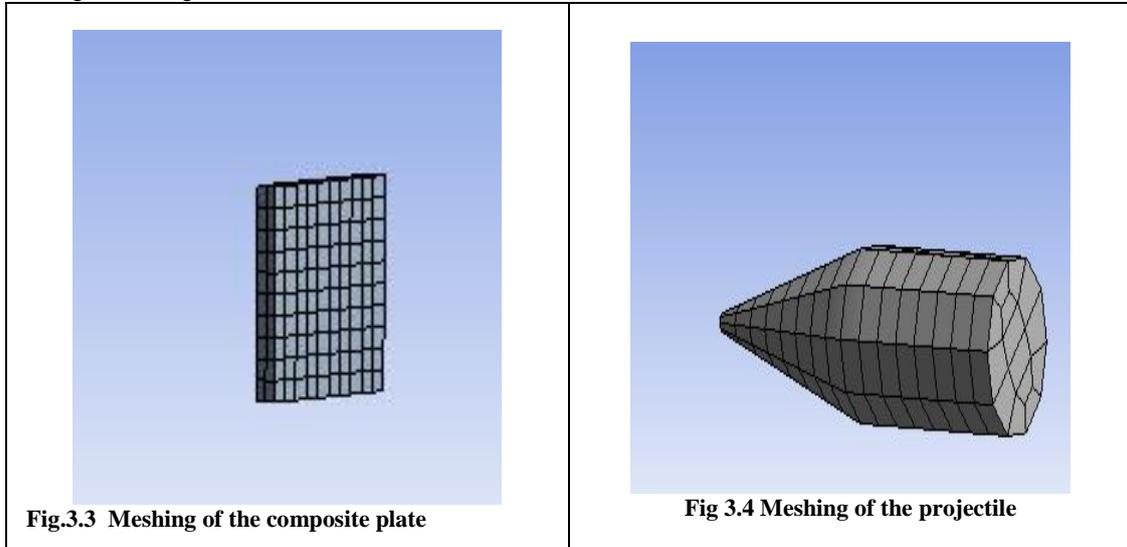
Fig.3.3 Meshing of the composite plate
