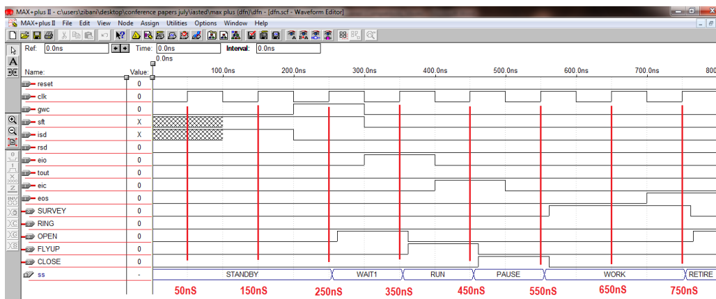
Figure 5. Simulation Waveform for DFN Control Unit. 8states x 2 8 input combinations!
