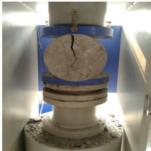
“Figure 2: Split tensile strength test specimen”
