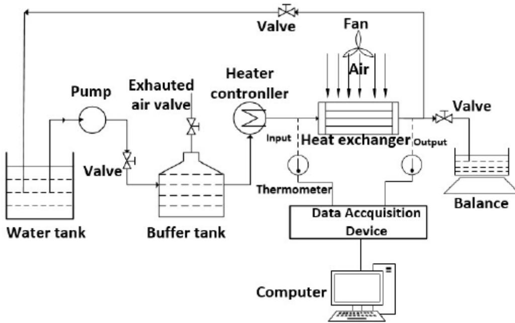
**Fig.3.** Schematic diagram of the test loop
