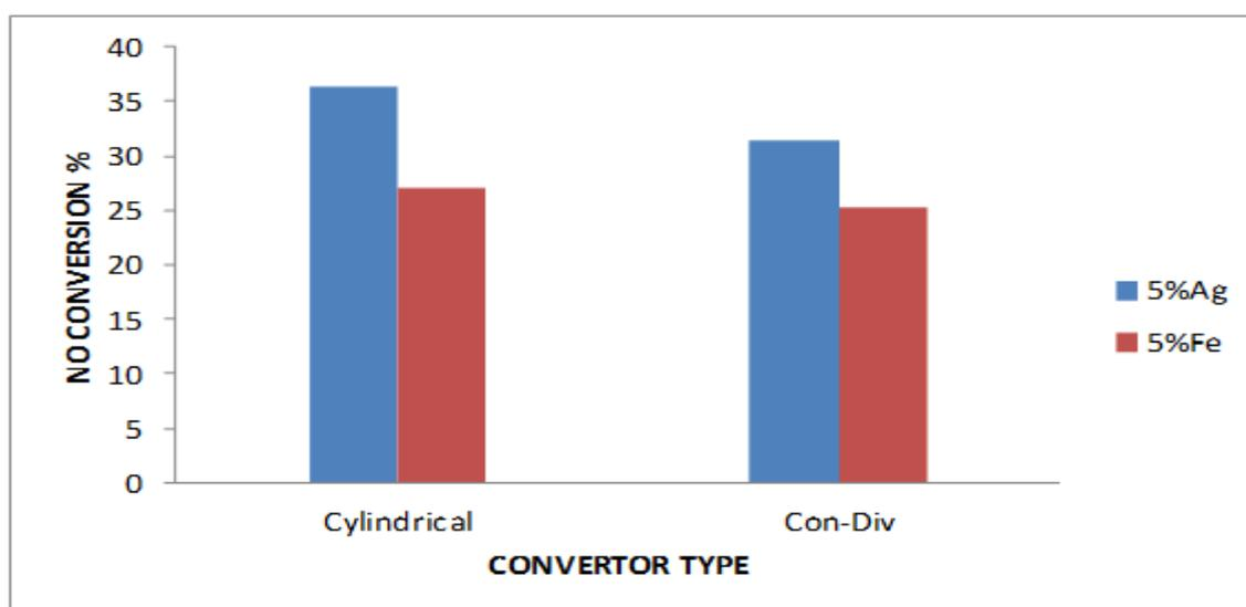
Fig 21: Type of catalytic converter V/s NO conversion%
