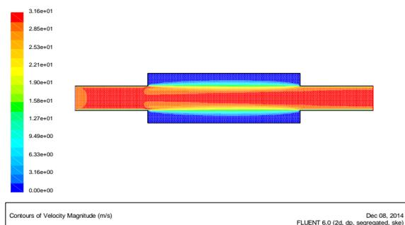
Fig 7 Velocity contour: Cylindrical Cat Con (Filled)
