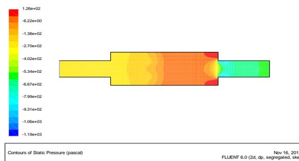
Fig 6 Pressure contour: Cylindrical Cat Con (Empty)
