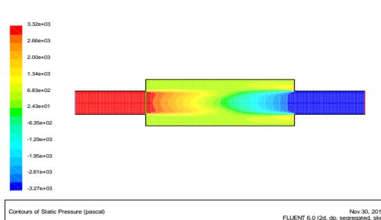
Fig 8 Pressure contour: Cylindrical Cat Con (Filled)
