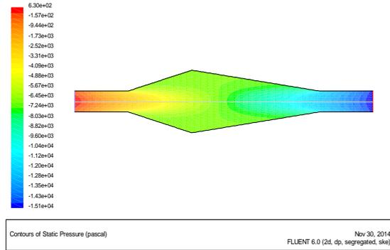
Fig 10 Pressure contour: Con- Div Cat Con (Empty)
