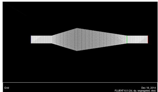
Fig 4 2D- Mesh file of Con-Div Catalytic Converter
