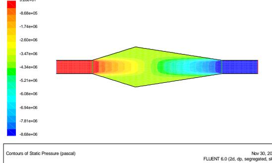
Fig 12 Pressure contour: Con-Div Cat Con (Filled)
