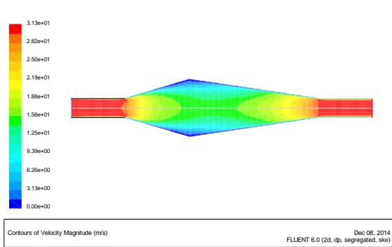
Fig 9 Velocity contour: Cov-Div Cat Con (Empty)
