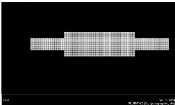
Fig 3 2D- Mesh file of Cylindrical Catalytic Converter
