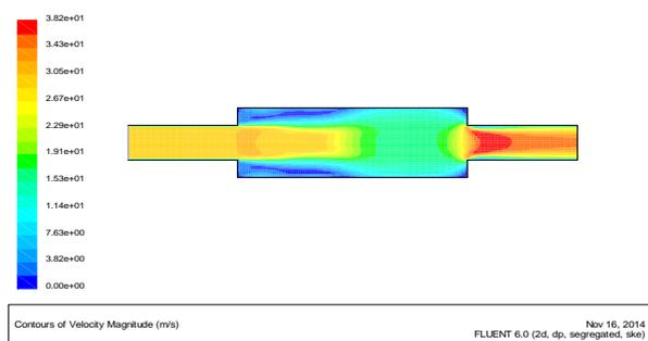
Fig 5 Velocity contour: Cylindrical Cat Con (Empty)
