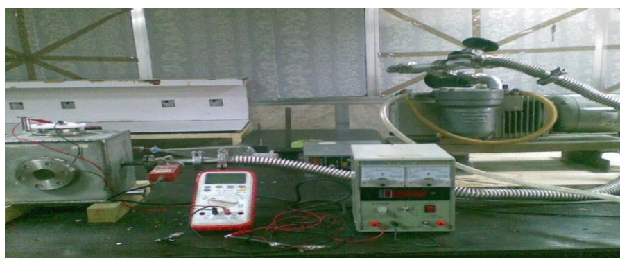
Figure (8) Experimental arrangement system for gas detecting
