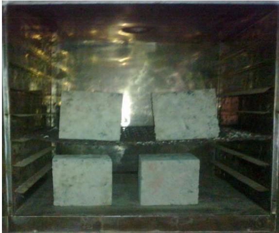
Fig-1: Specimens kept in Oven of 300°C capacity
