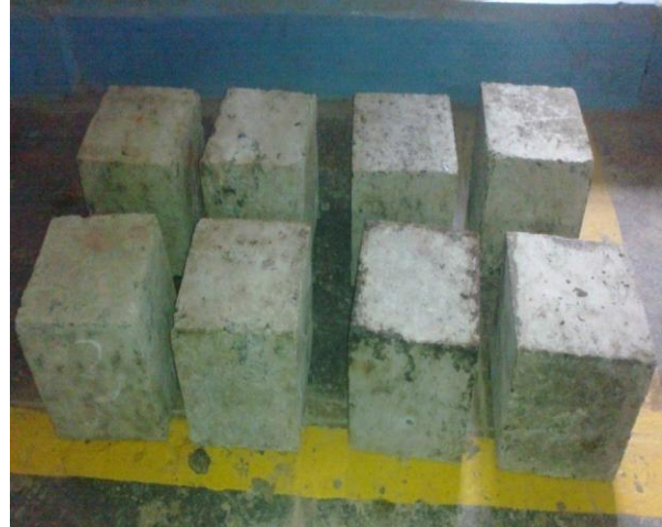
Fig-2 : Specimens kept at room temperature after removing from oven
