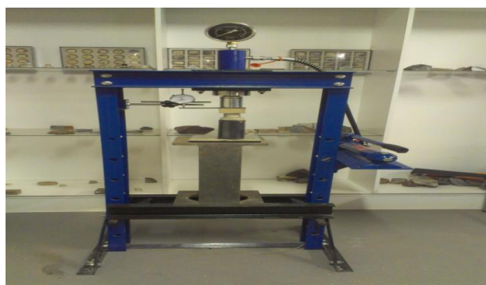
Fig. 2: Setup showing pre-loading stress applied after 12hours
