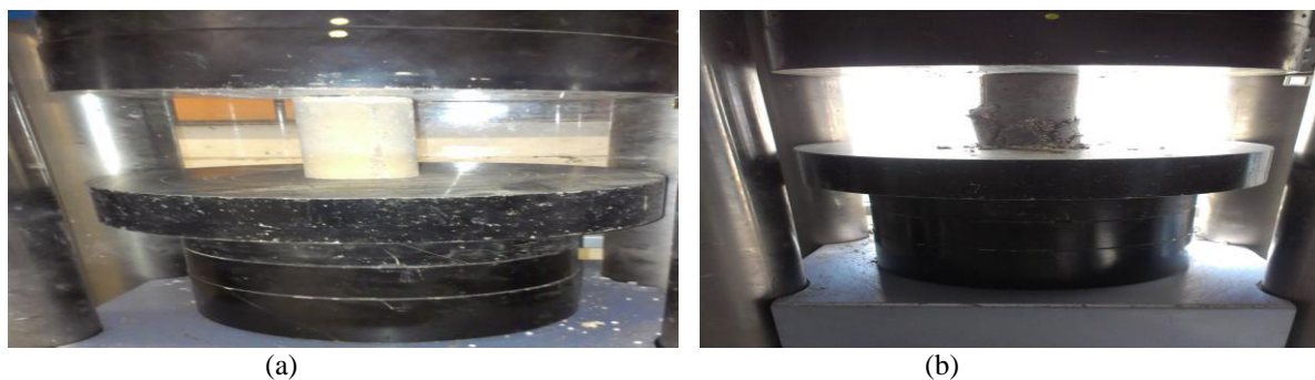
Fig. 6: (a) EPS-sand specimen underload (b) EPS-sand specimen failed from loading
