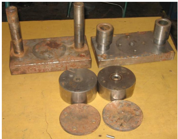
Fig 3 Tool and die set used in the present investigation
