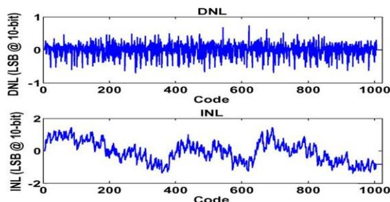
Fig.7 DNL and INL plot for 1.5 bit stage
