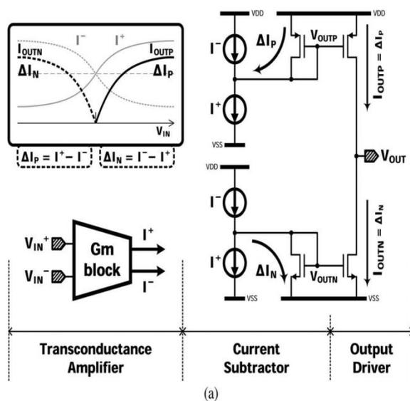
Fig. 3 Concept of the proposed Gm-based amplifier
