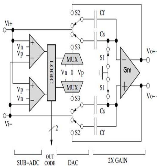
Fig.2 Simplified schematic of a 1.5-bit stage
