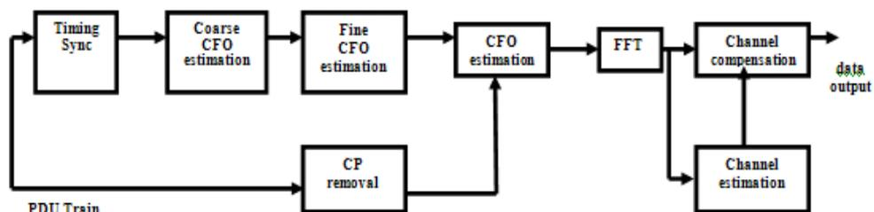
Figure 3. Receiver Structure
