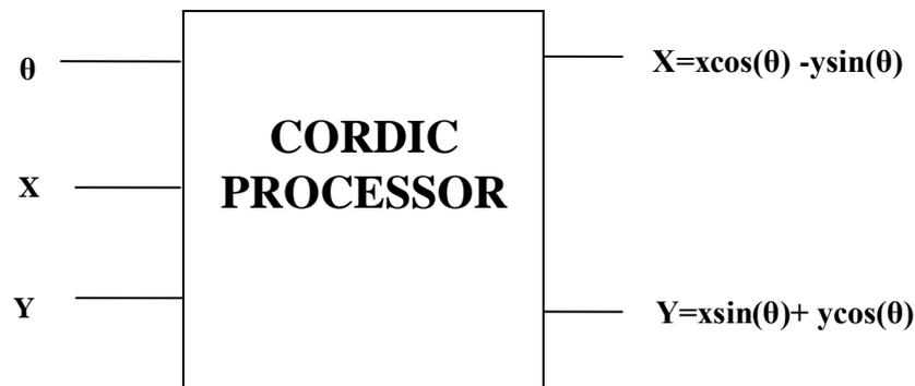
Figure 7. Block diagram of CORDIC Processor
