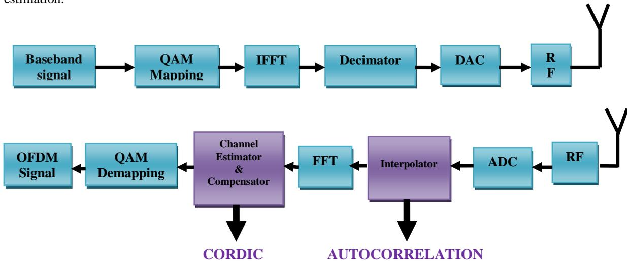
Figure 5. Block diagram of the proposed model
