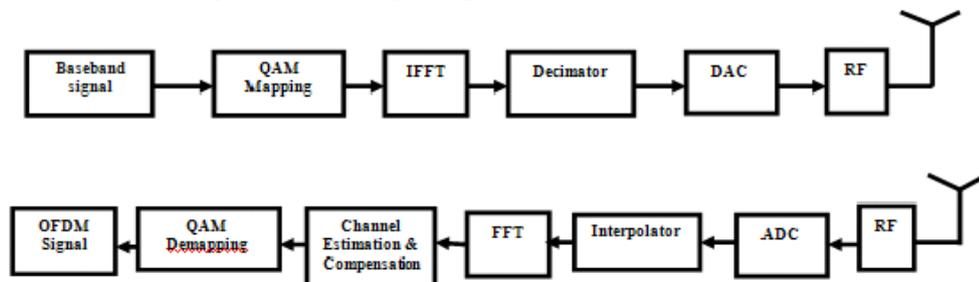
Figure 2. WLAN Transceiver
