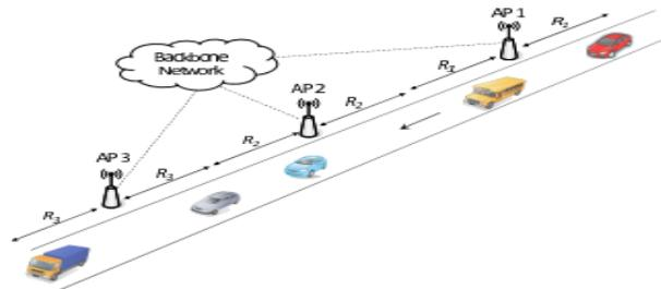
Fig. 1. Drive-thru vehicle-to-roadside (V2R) communications with multiple APs.
