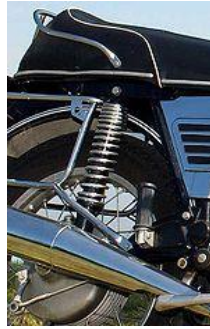
Fig.1: Rear shock absorber and spring of a BMW R75/5 motorcycle
