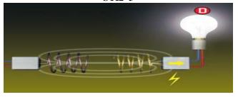
The energy of the oscillating magnetic field induces an electrical current in the receiving coil, lighting the bulb [D].
