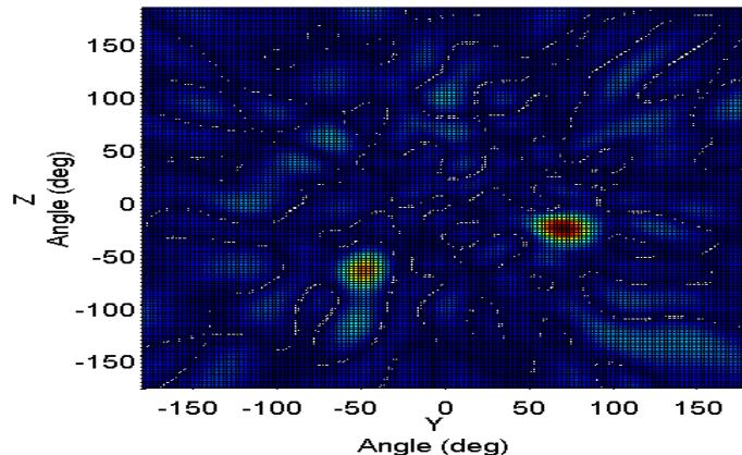
Figure.8. Maximizing the transmitted power around the targets of interest in the case of three false paths
