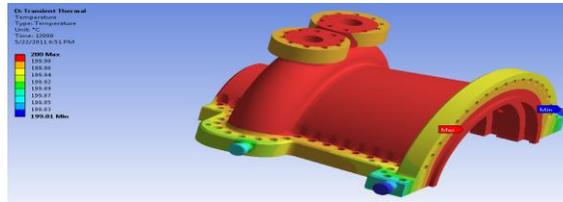
Fig43: Temperature Distribution in inner casing in unsteady (Transient) state condition after 12000s
