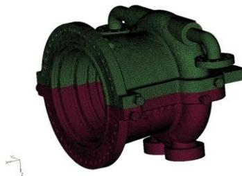
Fig 3.2: Steam Casing (HP) Meshed Model
