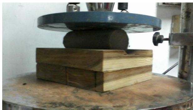
Split tensile strength of flyash with 5% lime and sodium silicate (free pouring consistency):
