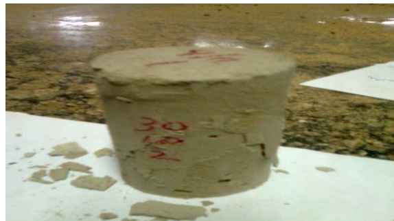
Unconfined Compressive strength of flyash with 5% lime and sodium silicate (free pouring consistency):
